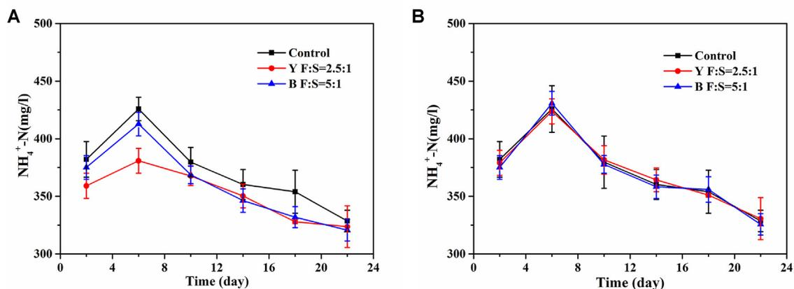
Fig. 7. TAN contents of the control, yellow, and black soil slurries. A: with  $Mg^{2+}$ ; B: without  $Mg^{2+}$ .
