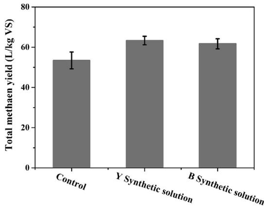
Fig. 5. Total methane production of the control, Y synthetic solution, and B synthetic solution.
