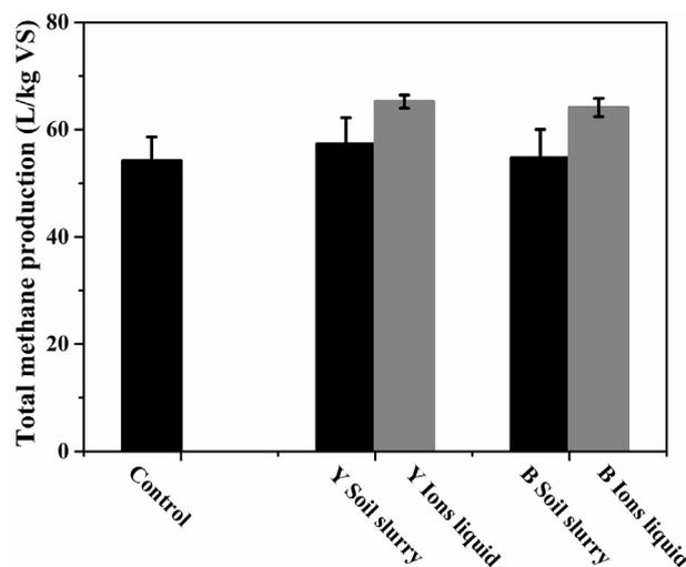
Fig. 4. Total methane production of the control, Y soil slurries, Y ion liquid, B soil slurry, and B ion liquid.
